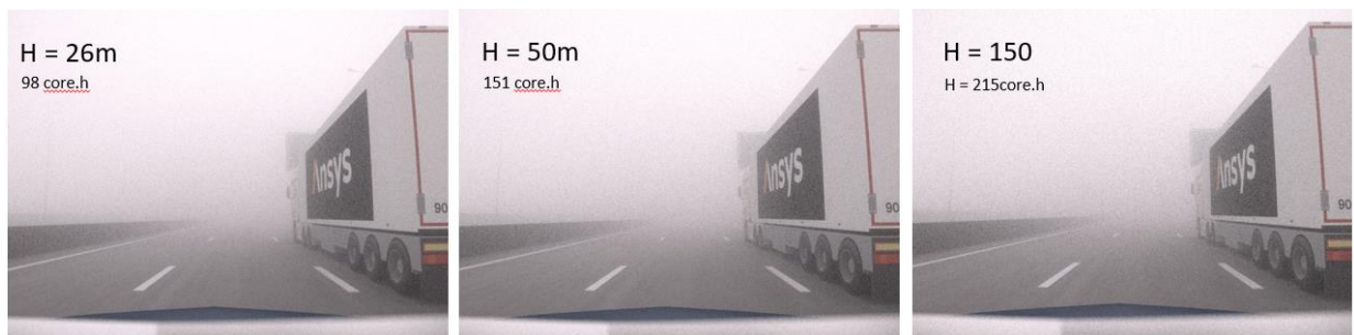
Figure 9 Influence of fog thickness on Camera visible simulations. Fog of visibility 50m.
