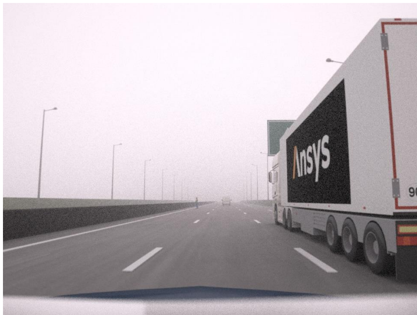
Figure 7 Ansys SPEOS simulation of pedestrian detection by a camera through fog. Fog is defined by a dome of 26m height and visibility v=150\text{m} from Duthon2019.
